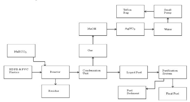
Figure 1: PVC and HDPE waste plastic mixture to fuel production process using NaHCO<sub>3</sub>
